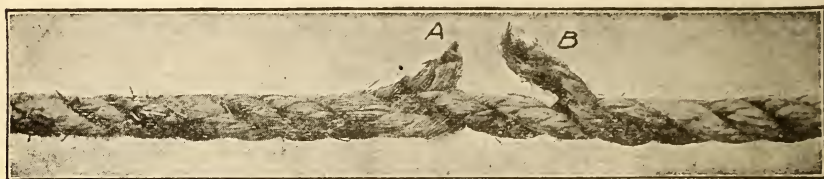
Fig. 1. A Broken Strand to Be Repaired.
